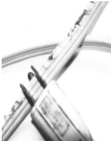
Fig. 1. (a) Electrical cord of a freezer in a retail market, severely damaged by house mice; (b) fiberglass batt insulation within walls of a hog finishing house near Lincoln, Nebraska, was destroyed by house mice in less than 3 years.
