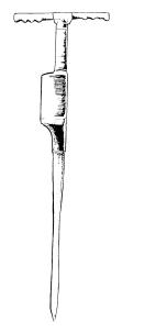
Fig. 8. Automatic bait dispensing probe for pocket gopher control.
