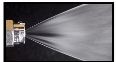
The **flooding (flat fan)** nozzle delivers a wide angle flat spray pattern. It operates at very low pressure and produces large spray droplets. Its pattern is fairly uniform across its width but not as even as the regular flat fan nozzle pattern. If used for broadcast spraying, it should be overlapped to provide double coverage. It is often used for applying liquid fertilizers or fertilizer/pesticide mixtures.
