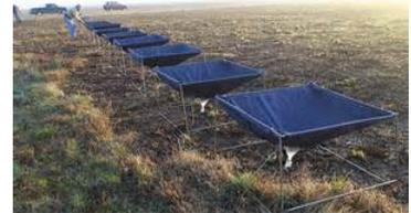
Fly a swath test along a centerline oriented at a right angle to the line of collection pans. If ambient wind speed is greater than a sustained 8 mph, orient the line of pans at a right angle to the prevailing wind and fly directly into the wind.
