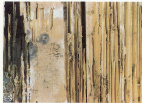
Figure 7. — Wood attacked by subterranean termites has a honeycombed appearance because the workers tunnel along the softer grain of the wood.
