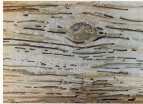
Figure 6. — Surface of wood removed to show damage done by termites and the specks of excrement on the gallery walls.
