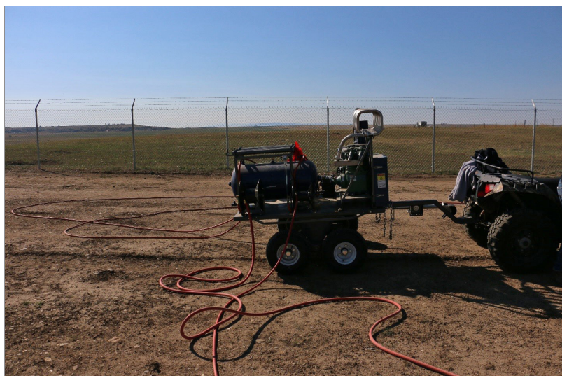
FIGURE 6.15. P.E.R.C.® device with three hoses being used on a prairie dog town. Photo by Stephen M. Vantassel, MDA.
