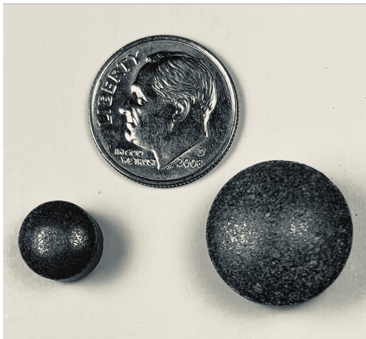
FIGURE 2.4. An aluminum phosphide pellet (left) and tablet (right). Photo by Stephen M. Vantassel, Montana Department of Agriculture (MDA).
