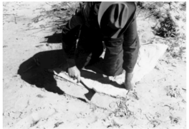
Fig. 10. Kneel down on the cloth and outline a trench approximately 3 feet long, 7 inches wide, and 2 inches deep. Dig the trench so that it runs lengthwise to the prevailing wind.
