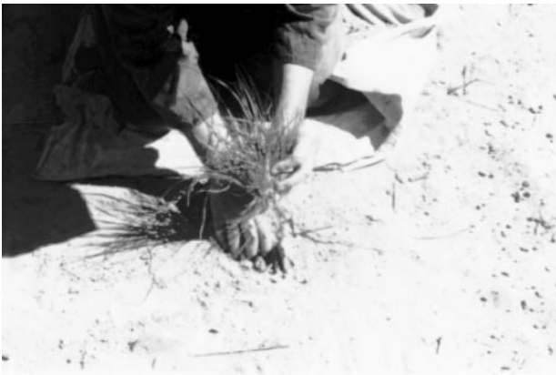
Fig. 24. Place an object over the buried stake that can be easily seen; the further away it can be seen, the better. Use an old, dried bleached bone, a dried cow chip, a small bush or clump of grass, an old dried root, a small stake, or a stump. The object should be about 6 to 8 inches high and be very visible.
