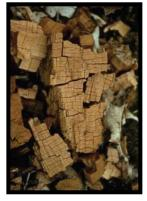
Brown rot in a dry, crumbly condition is sometimes incorrectly referred to as "Dry Rot" as wood must be moist to decay. This term is used because the features described above become most apparent after the wood has dried, thus the term "dry-rot" has been incorrectly used to describe the condition. Brown Rot fungi are the major cause of decay of wood products in Nevada.
