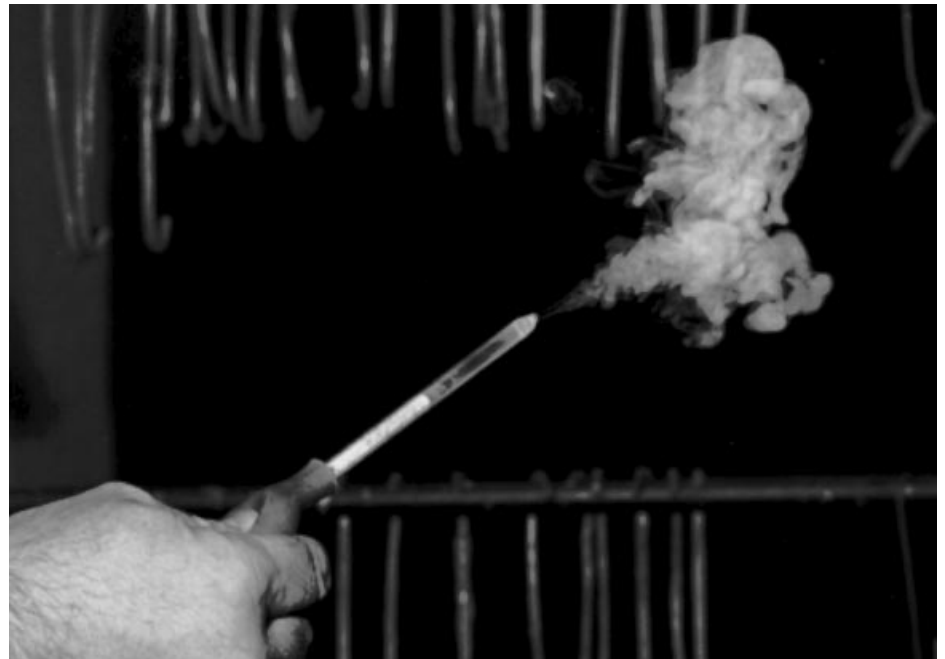
Fig. 11. Smoke from the Sensidyne Air Indicator makes it possible to visually determine the directional pattern of air currents.
