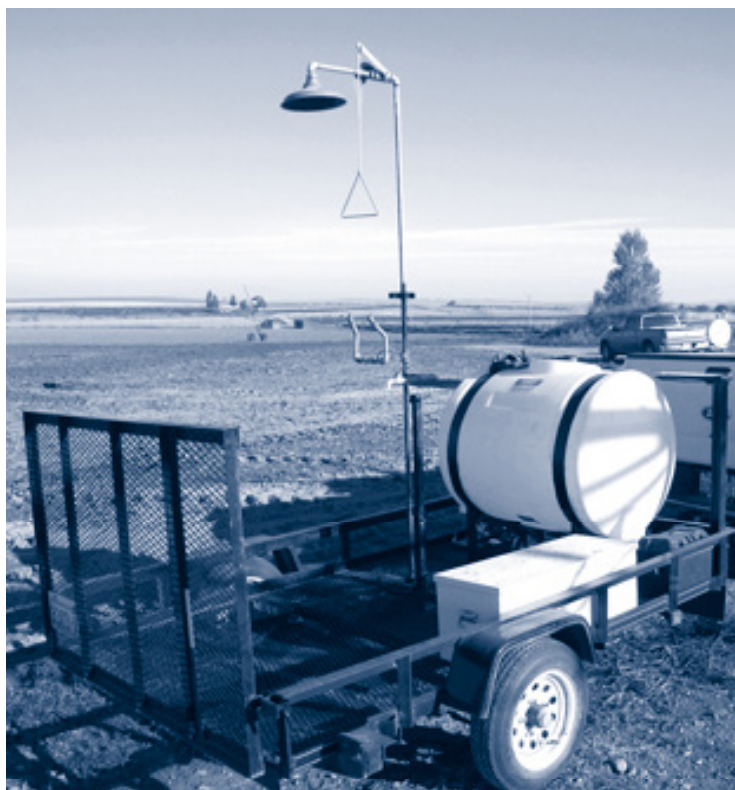
Portable decontamination unit
